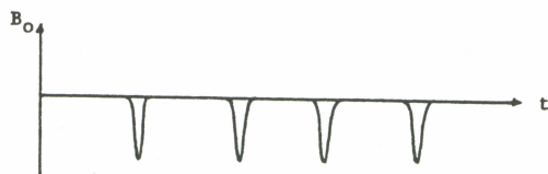
Fig. 3 The resonance condition is signaled by an enhanced attenuation of the radio waves passing through the sample.
